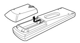
2. Insert batteries. Make sure to match the polarity: (+) to (+) and (-) to (-).
