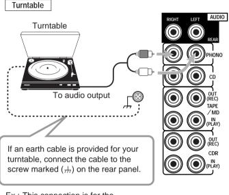
Ex.: This connection is for the turntable with an MM (moving-magnet) type cartridge.
