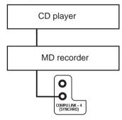
2) TEXT COMPU LINK jacks: Use the cables with the stereo mini-plugs (not supplied with this receiver).
