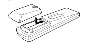
If the range or effectiveness of the remote control decreases, replace the batteries. Use two R6P(SUM-3)/AA(15F) type dry-cell batteries.
